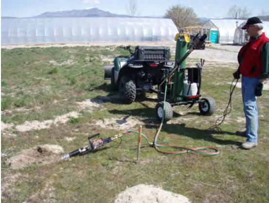
A truly effective, poison and pesticide-free method of eliminating burrowing rodents called the Rodenator.
